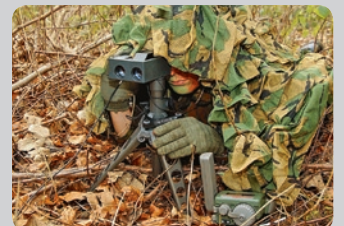
Placing the PLRF on a tripod facilitates the lasing of small, distant objects of feeble reflectivity. Measurements are released using the remote trigger on the optional data cable.
