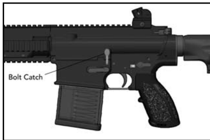
Fig. 18 – Depressing Bolt Catch to Chamber a Cartridge
