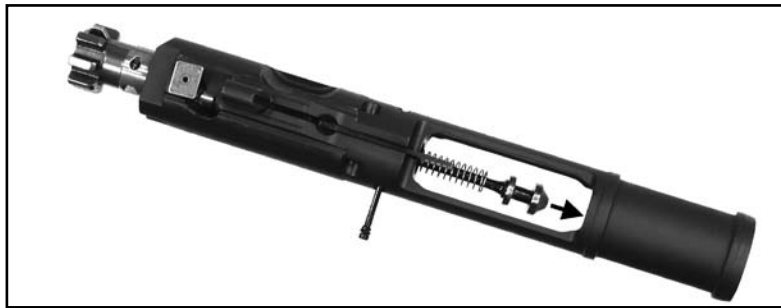
Fig. 26 – Removing the Firing Pin and Firing Pin Spring from the Bolt Assembly
