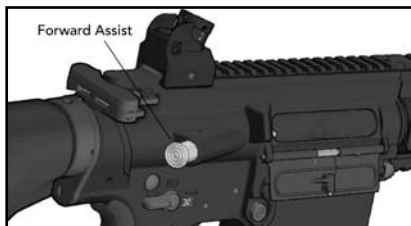
Fig. 19 – Tap Forward Assist
