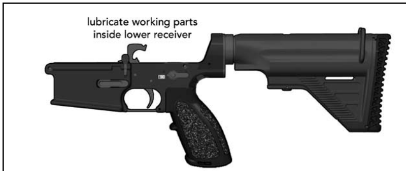
Fig. 59 – Lubrication of MR762A1 Lower Receiver Assembly
