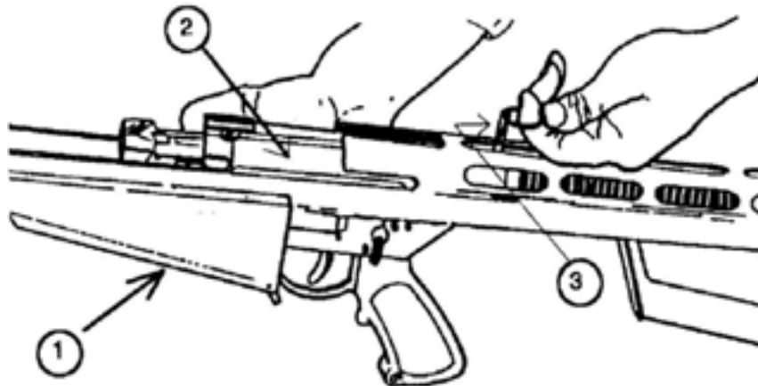
Figure 2-7. Releasing Bolt Carrier From Storage Configuration
