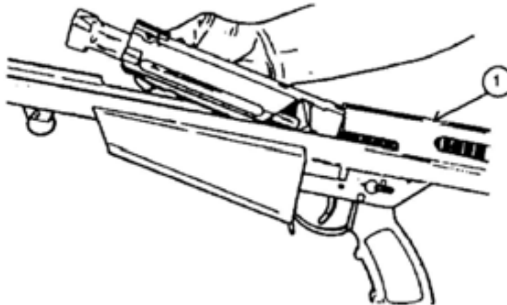
Figure 2-15. Removing Bolt Carrier From Storage Configuration
