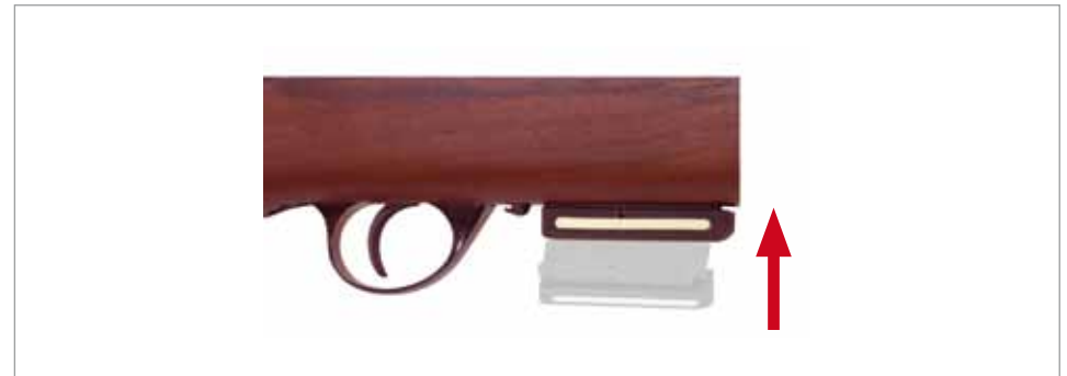
Fig.5 Inserting the magazine
