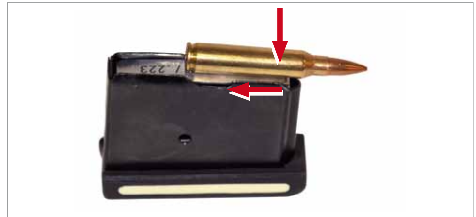
Fig.3 Loading the magazine
